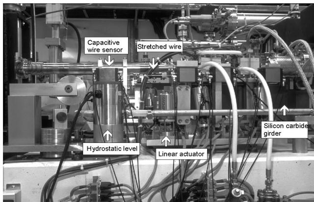
Figure 5: End station of the stretched wire system.
