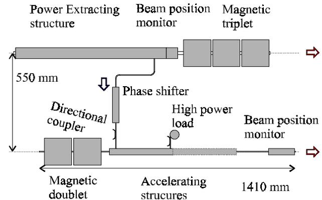
Figure 1: Schematic layout of one module of the main (lower) and drive (upper) linacs.
