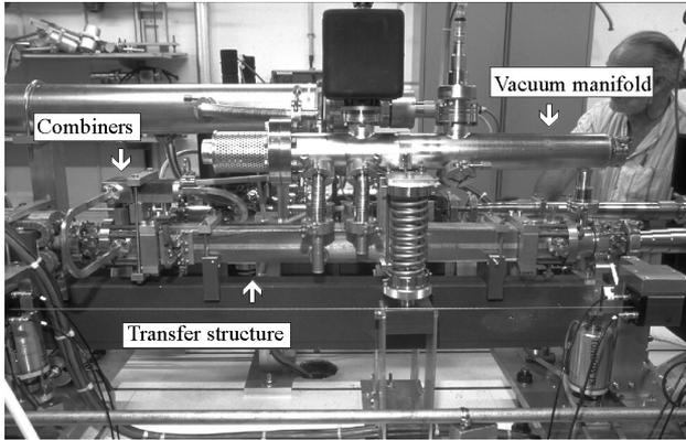
Figure 3: Installation around a power extracting structure.
