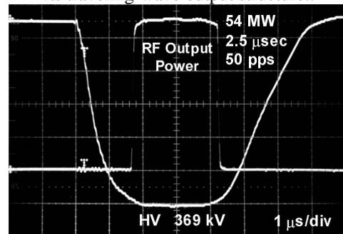
Fig. 6 RF output power of the second E3746 C-band klystron.
