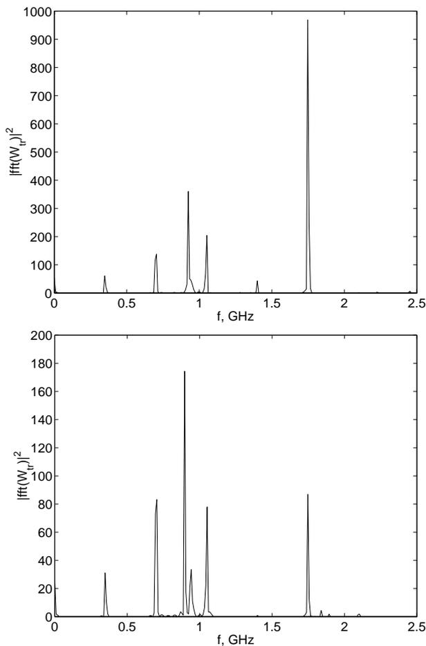
Figure 3: Power spectra of the transverse wake potentials for 30 bunches in the APT 5-cell cavities:  $\beta = 0.64$  (top) and  $\beta = 0.82$  (bottom).
