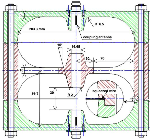
Fig. 2. Longitudinal section (transverse view on fig.4)
