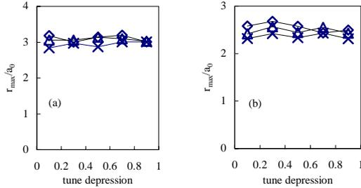
Figure 5: Ratio of the maximal radial extent to radius of matched beam vs  $\eta$  for mismatch parameter (a)  $\mu=0.6$ , (b)  $\mu=0.8$ , with different  $\sigma_0$ :  $\diamond-85^\circ$ ,  $\Delta-75^\circ$ ,  $\times-65^\circ$ .
