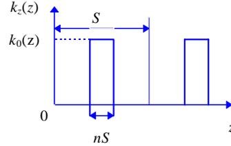
Figure 1: The profile of solenoidal periodic focusing field
