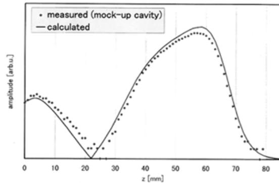
Fig. 9. Measured and calculated longitudinal field profile
