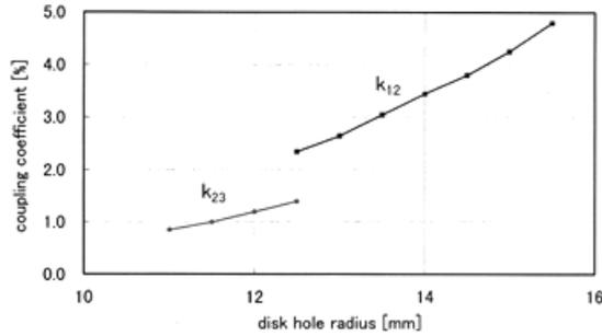
Fig. 3. Disk hole radii vs. coupling coefficients
