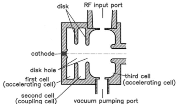
Fig. 1. Cross sectional view of OCS type RF gun
