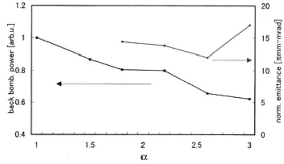
Fig. 4. Field balance (a) vs. beam emittance and back bombarding power
