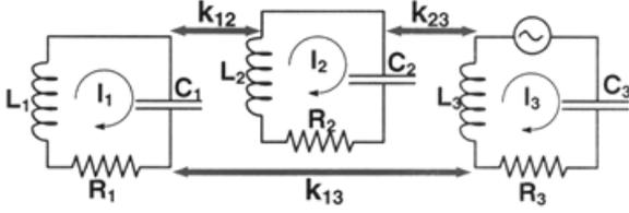
Fig. 2. Coupled resonator model for OCS type RF gun
