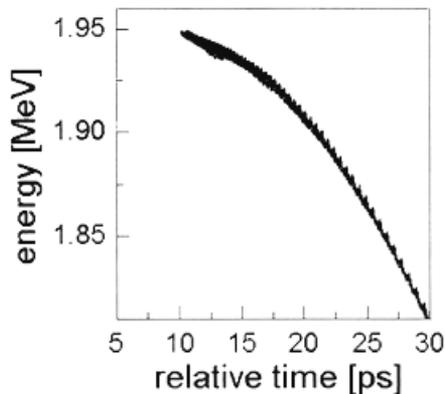
Fig. 8. Time dependence of energy of output beam
