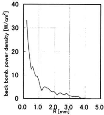
Fig. 6. Radial distribution of back bombarding power density
