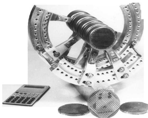
Fig.2. Space lattice electrodes and their possible arrangement in RF structure
