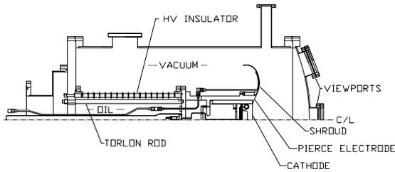
Figure 2: An assembly drawing of the gun and vacuum test chamber.
