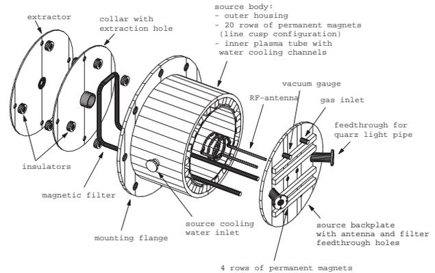
Figure 1: Ion Source Cross Section
