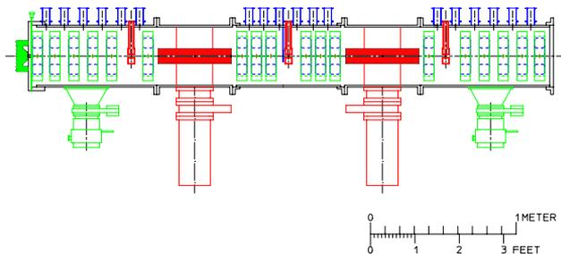
Figure 5: MEBT in Common Vacuum Chamber
