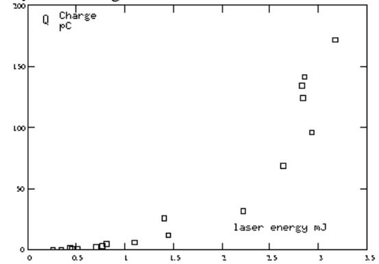
Figure 5: Emission versus laser energy for a PLZT 4/95/5 sample when the applied voltage was 7 kV.
