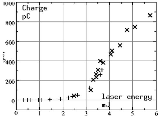
Figure 2: Emitted charge versus laser energy for a PLZT 8/65/35 without the front grid. Notice the clear bending of the curve due to the space charge effect.
