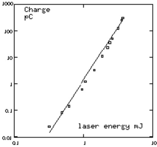
Figure 3: Emitted charge versus laser energy for a PLZT 8/65/35 without the front grid in log-log frame. The continuous line is a fit with  $Q \propto I^4$  scaling law.
