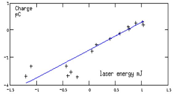
Figure 4: Emitted charge versus laser energy in logarithmic scale for a PLZT 4/95/5 sample when the applied voltage through the gap was 3.5 kV. The continuous line fits with  $Q \propto I^2$  scaling law.
