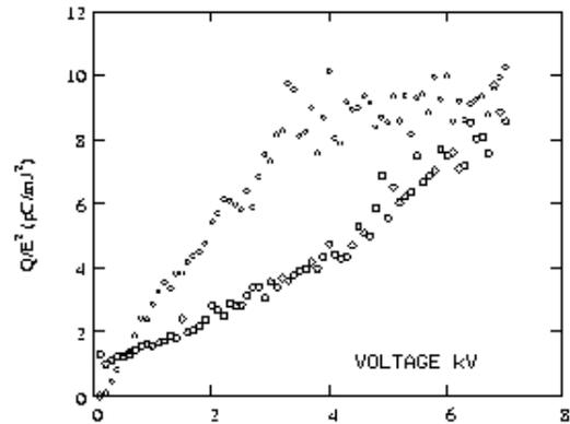
Figure 6: Emitted charge versus laser energy: the lower points are obtained at 7 kV of applied voltage, while the points of the upper curve are obtained in succession but after having reduced the voltage to 3.5 kV. The hysteric behavior was not observed keeping constant the voltage.
