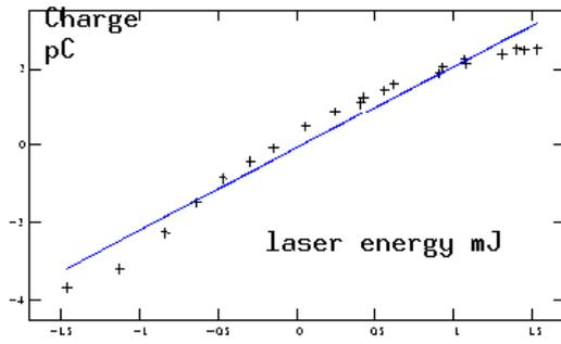
Figure 7: Charge versus laser energy in log-log scale for PT. The continuous line fits with  $Q \propto I^2$  scaling law.
