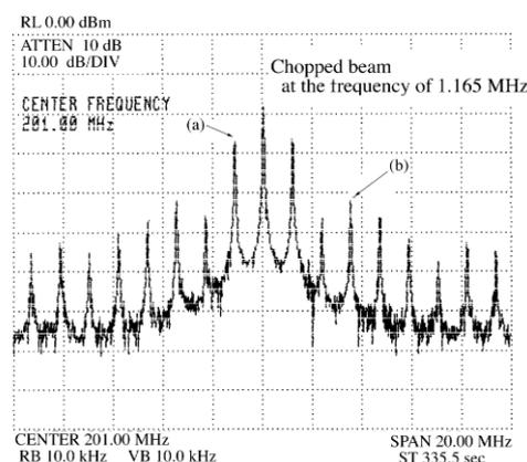
Fig. 1 Frequency components of chopped beams. Chopped beams were produced by using a beam-chopping system developed at KEK. An average beam intensity was about 8 mA. The post-1 and TM012-modes were excited by the frequency components of (a) and (b), respectively.
