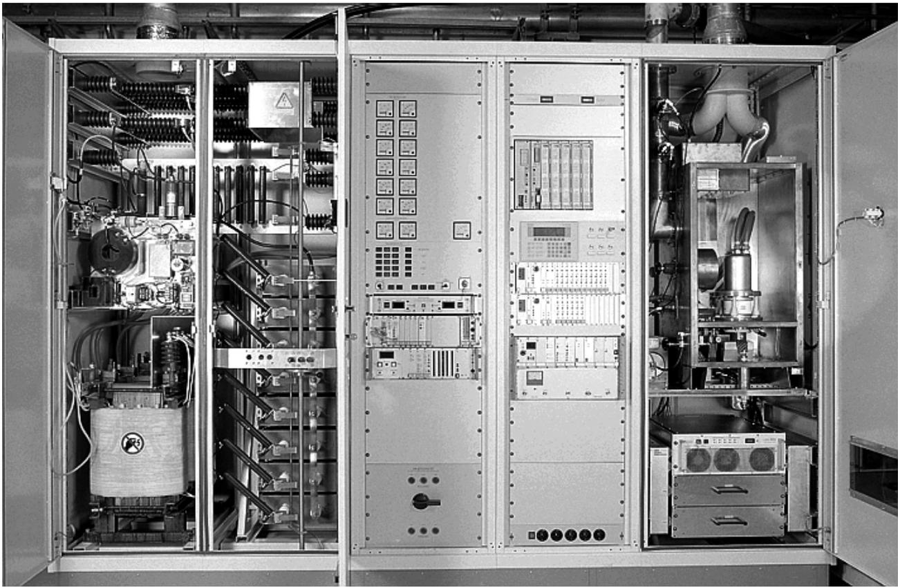
Fig. 3 : Front View of the 200 kW / 36 MHz Amplifier (by Thomcast AG) : the plate supply (two cabinets left); the local operation panel with computer interface and plunger control (3<sup>rd</sup> cabinet); Program controlled computer [Simatic] with the measuring device and amplitude & phase controls (4<sup>th</sup> cabinet); opened anode & grid circuit of the 200 kW stage with the 2 kW solid state amplifier (by Dressler) and the tube grid supplies below (right cabinet)
