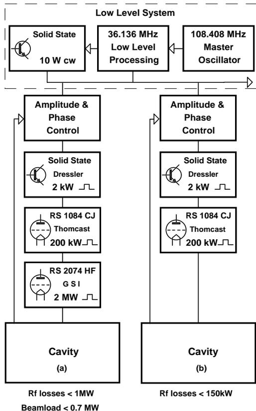
Fig. 1: Amplifier Chains of the New High Current Injector: (a) RFQ, IH1-DTL and IH2-DTL, (b) Superlense and Buncher
