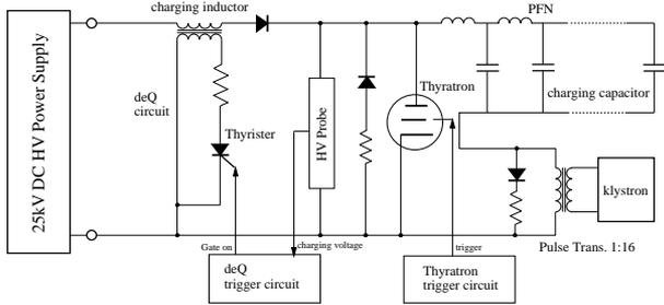
Figure 1: The simplified diagram of the modulator
