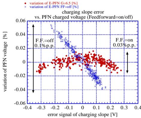
Figure 5: correlation between a charging voltage slope and charged voltage equilibrium with feedforward on/off
