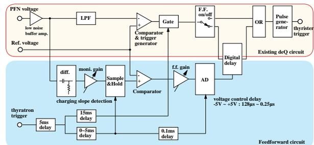
Figure 4: The block diagram of the feedforward circuitry
