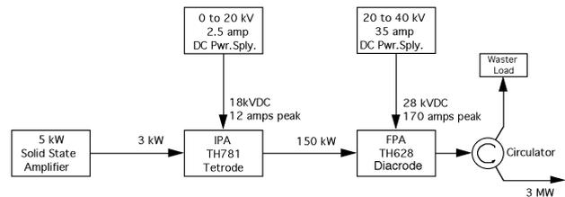
Figure 2. New configuration for RF modules 3 and 4
