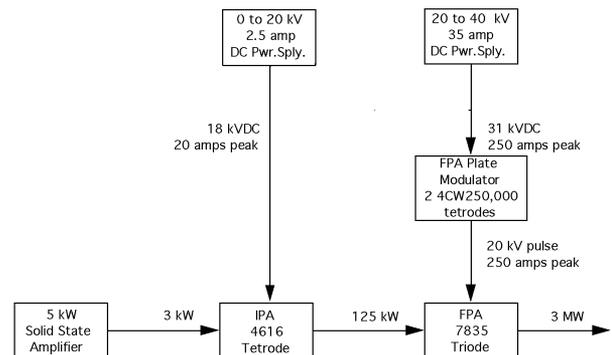
Figure 1. Present configuration - high power RF modules
