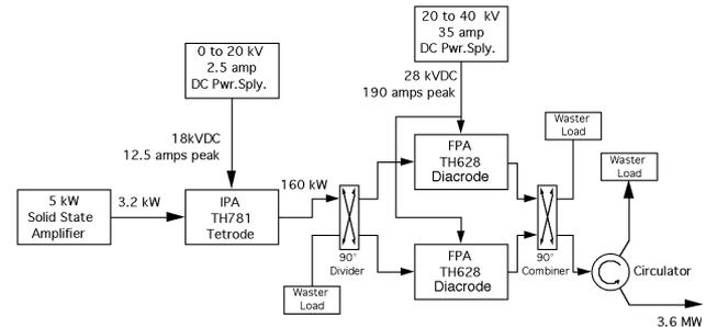
Figure 3. New configuration for RF module 2
