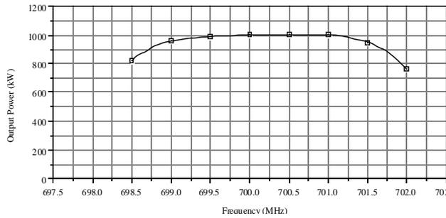
Figure 4: CPI klystron frequency response.
