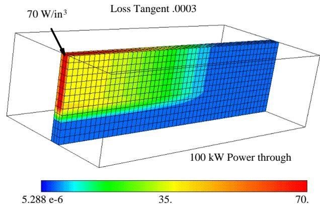
Figure 3: Heat loss contours determined by MAFIA
