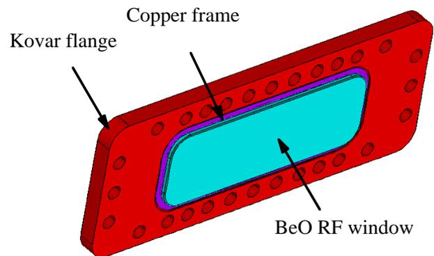
Figure 1: BeO RF Window, Flange and Frame
