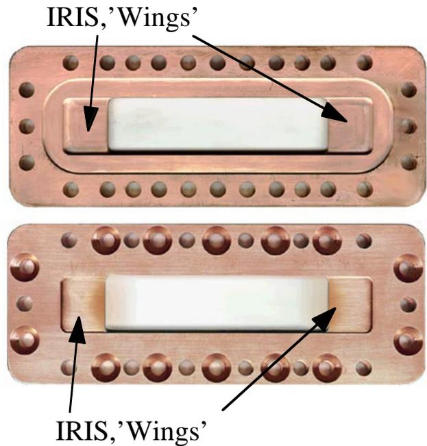
Figure 2: RF window and Iris('wings') and flange
