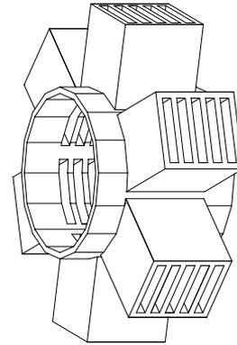
Figure 1: Schematic drawing of the waveguide array absorber.
