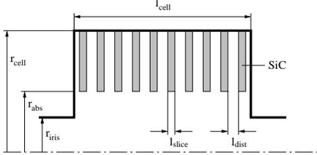
Figure 3: Laminated SiC absorber.
