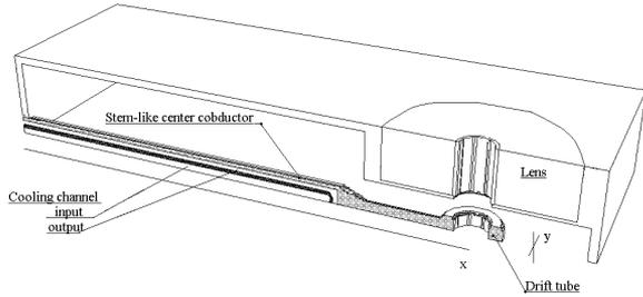
Figure 2: The double-gap bunching cavity with the straight central conductor
