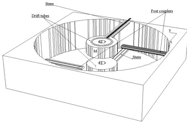
Figure 1: A sketch of DTL structure
