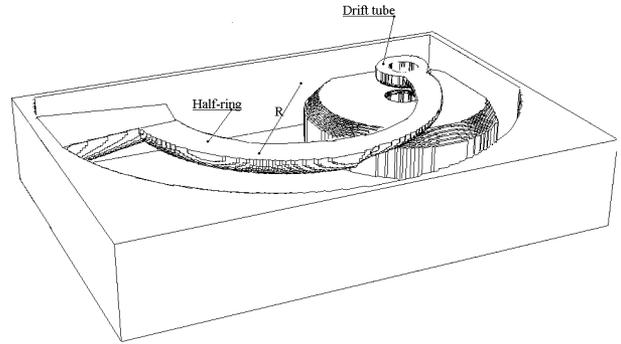
Figure 3: The double-gap bunching cavity with the ring central conductor
