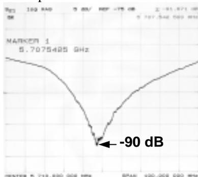
Figure 6: Frequency response of choke cavity.
