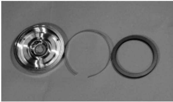
Figure 5: An SiC rf absorber components. Left: choke-mode cavity. Center: metal spring belt. Right: SiC rf absorber ring. An SiC rf-absorber ring is inserted smoothly into the outer groove by using a simple jig with pressure around 30 kgf.
