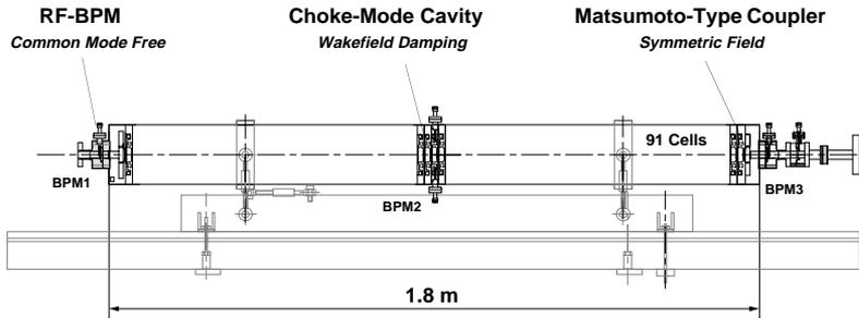
Figure 3: 1.8 m long high power C-band choke-mode structure.
