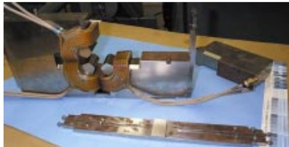
Because of the large number of magnets, and the overall congestion of all areas around the beam line, alignment of the magnets after installation could be a problem. For this, and to minimize personnel radiation exposure, we will be pre-aligning all of the magnets off-line, to a common standard, on semi-kinematic mounts. The calibration and pre-alignment standard has been designed, and is being assembled by General Atomics.
