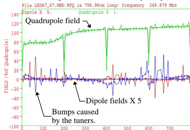
Figure 1. RFQ fields measured with the bead perturbation technique. The measured fields are within 1% of the design values. The dipole fields are multiplied by a factor of 5.
