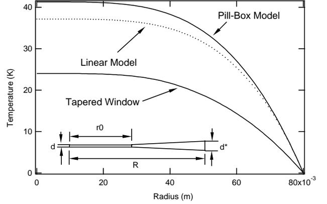
Figure 3: Temperature distribution on a flat Be window with thickness of 0.127 mm and on a tapered window with  $d^* = 0.254$  mm. Note the temperature difference of  $T(0) - T(R)$  is plotted here.  $T(0) \approx 77$  K and  $T(R) \approx 300$  K for the LN and room temperature, respectively. The temperature raise of the tapered window is about 15 K lower than the flat one.
