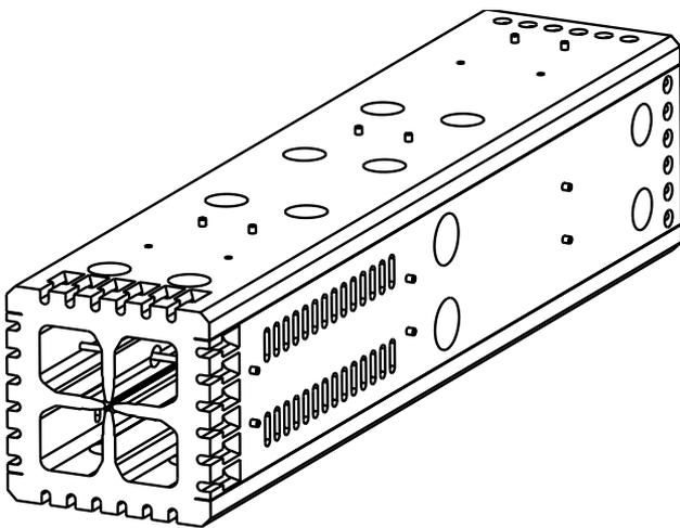
Figure 1 - Schematic view of one RFQ module
