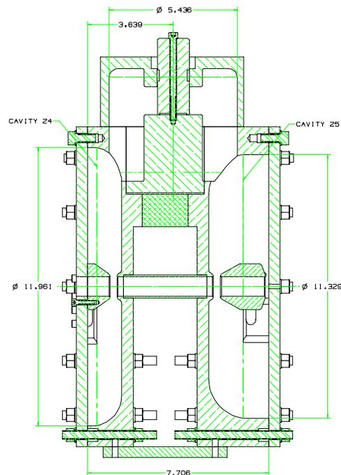
Figure 1: Drawing of transition region cold model.
