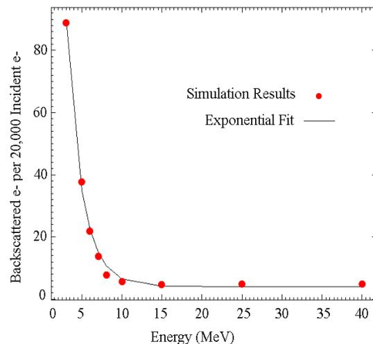
Figure 1: Number of backscattered electrons versus incident beam energy with a superimposed exponential fit.
