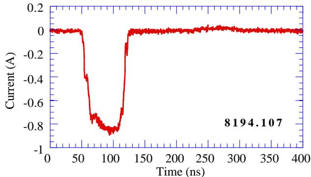
Figure 3. Typical output from the forward faraday cup.
