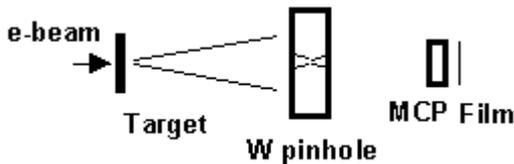
Figure 2. X-ray pinhole camera.
