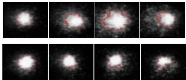
Figure 3. Time resolved x-ray spot comparison between 15° off normal (top) and normal incidence (bottom).
