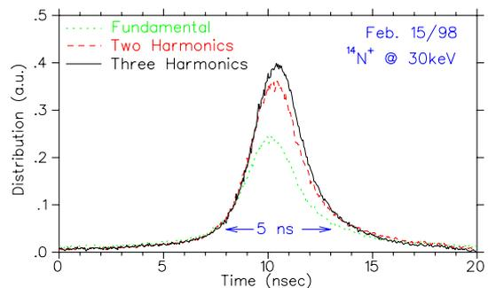
Figure 4: Beam bunches measured on the fast Faraday cup in LEBT for one, two or three harmonic bunching.
