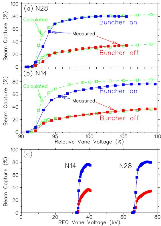
Figure 5: RFQ beam test results showing capture efficiency as a function of relative vane voltage for (a)  $N_{28}^+$  and (b)  $N_{14}^+$ . The nominal vane voltage in each case was 71.9 kV and 36 kV respectively. The beam capture for both bunched and unbunched initial beams are recorded (solid line) and are compared with PARMTEQ calculations (dashed lines). In (c) the results are plotted with respect to absolute vane voltage.
