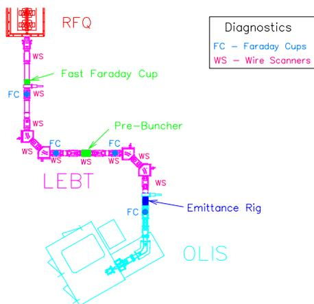
Figure 3: The layout of the off-line ion source (OLIS) and low energy beam transport (LEBT) upstream of the RFQ. The commissioning diagnostics are indicated.
