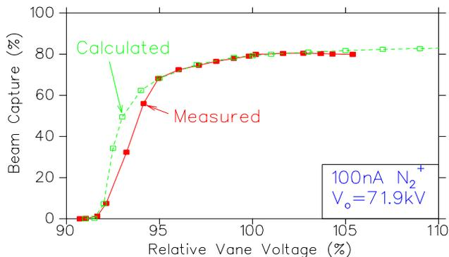
Figure 3: Beam test results from the RFQ. Shown is the capture efficiency of a  $N_2^+$  beam as a function of relative vane voltage (solid line). The calculated capture efficiency is plotted (dashed line) for comparison.
