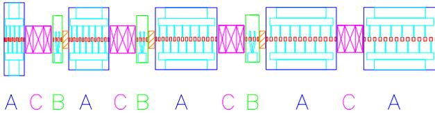
Figure 4: Schematic drawing of the ISAC variable energy separated function DTL. Five IH tanks (A) provide acceleration at  $0^\circ$  synchronous phase, three triple gap spiral resonators (B) provide longitudinal focus ( $\phi_s \sim -60^\circ$ ) and quadrupole triplets (C) provide transverse focus.
