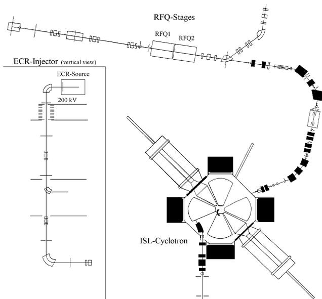
Figure 1: Scheme of the beamline
