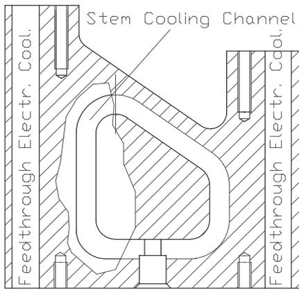
Figure 6: Cooling of the endstem with split water flow.
