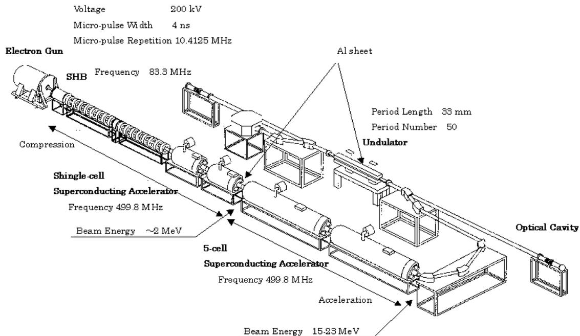
Figure 1: Schematic Layout of the JAERI Superconducting Linac
