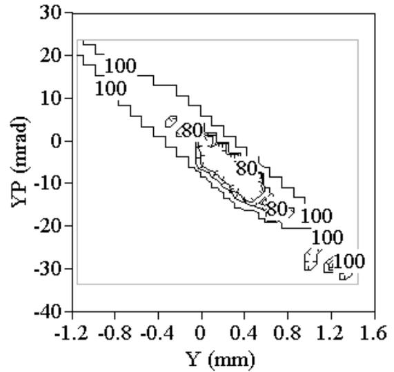
Figure 4: Reconstructed phase space contour of 100 % and 80 % emittance.
