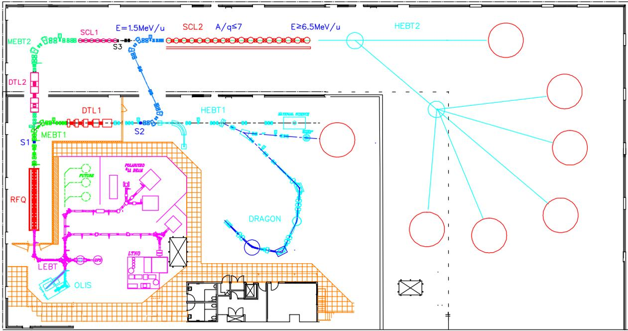
Figure 1: ISAC2 layout, including link from ISAC1, as would be needed for a 2-stripper stage
