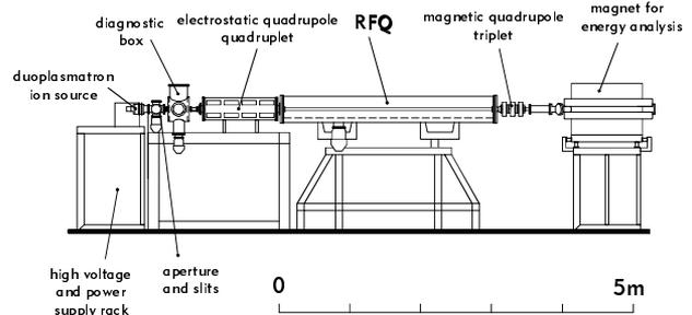
Figure 5: Lay-out of REX-ISOLDE test beam line for beam analysis of the RFQ beam
