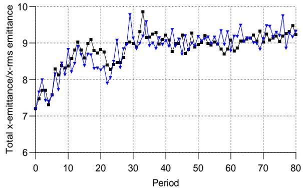
Figure 3: 99.9% total to rms emittance ratio for a matched (squared) and a high mode excited case (triangles)
