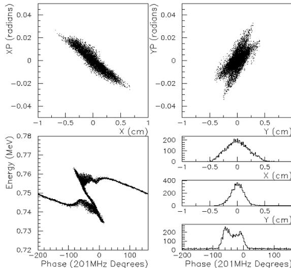
Figure 2: The simulated transverse and longitudinal  $H^-$  beam distributions at injection to the DTL.
