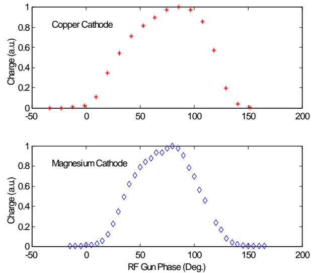
Figure 3: Photoelectron charge as function of RF gun phase for different cathode materials.
