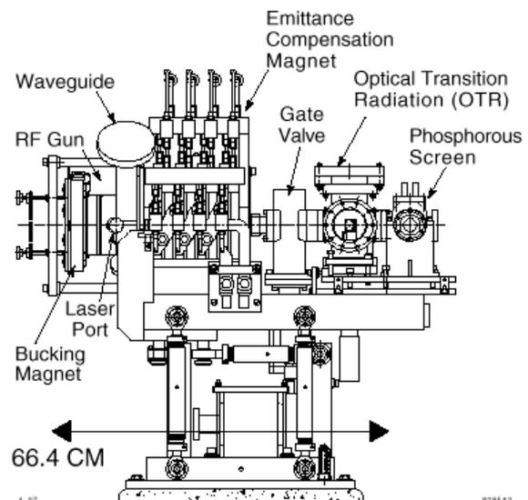
Figure 1: Layout of the ATF photoinjector.
