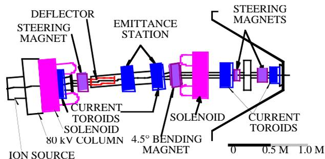
Figure 1. Schematic depiction of the major components of the 80 keV beam transport inside the LANSCE H<sup>-</sup> Ion Injector.
