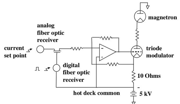
Figure 2. Magnetron current-modulator diagram.
