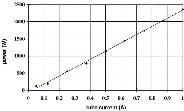
Figure 3. Microwave power versus tube current.
