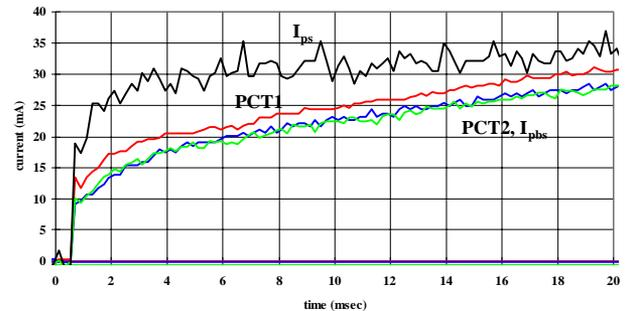
Figure 7. Leading edge of the beam current extracted from the 50-kV triode injector.
