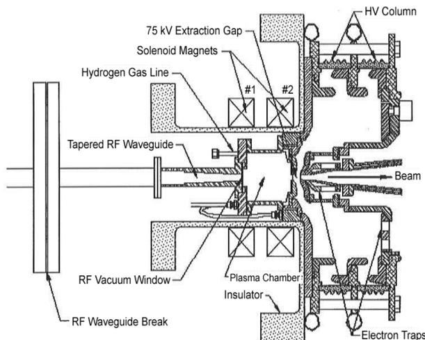
Figure 1. LEDA microwave proton source.
