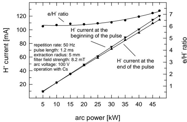
Figure 3: H<sup>+</sup> current and e/H<sup>+</sup> ratio vs the arc power.
