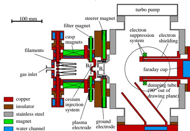
Figure 1: Schematic drawing of the experimental setup.
