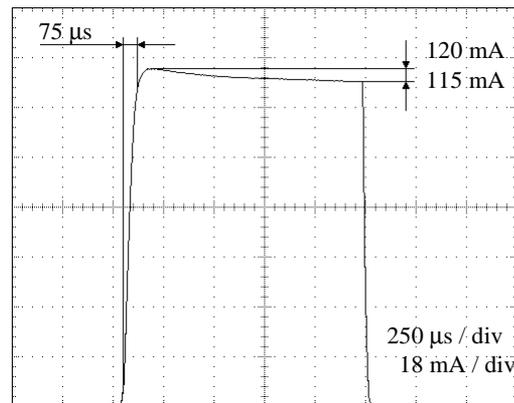
Figure 4: Oscillogram of the H<sup>+</sup> beam.
