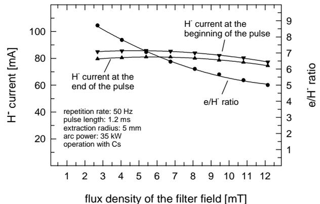
Figure 5: H<sup>+</sup> current and e/H<sup>+</sup> ratio vs filter field strength.
