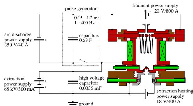
Figure 2: Wiring diagram of the  $H^-$  ion source.
