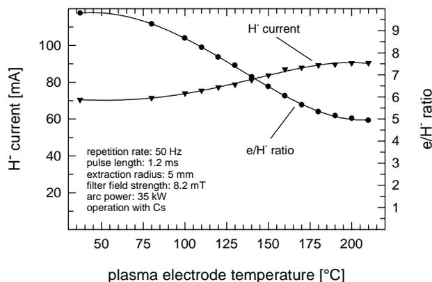
Figure 6: H<sup>+</sup> current and e/H<sup>+</sup> ratio vs plasma electrode temperature.
