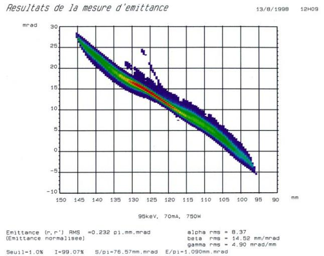
Figure 2 : Typical measurement with the reference EMU.
