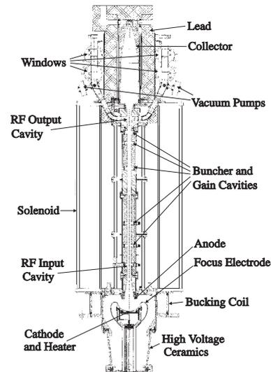
Figure 1: Layout of klystron #1
