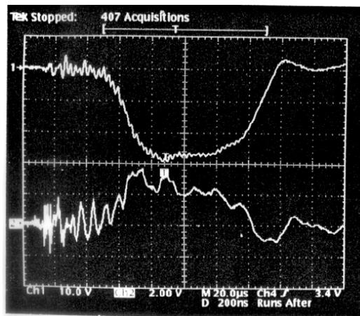
Figure 5. Output pulse waveform at the resistor load.
