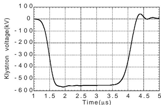
Figure 3. Output pulse waveform simulated by a computer code Micro-Cap IV.
