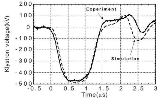
Figure 2. Output pulse waveform at the klystron.
