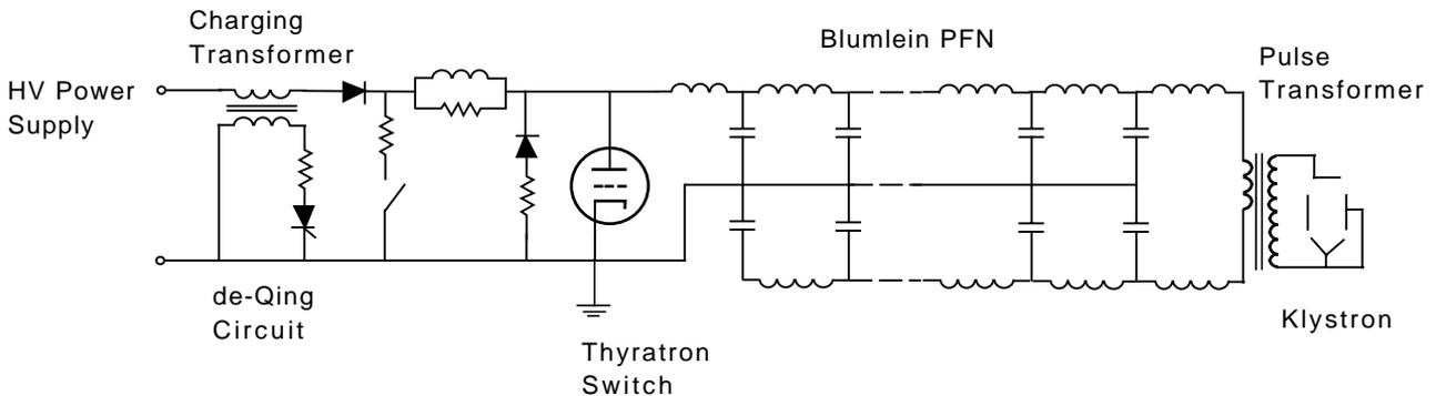
Figure 1. Circuit of the Blumlein type modulator.
