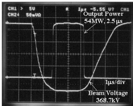
Figure 3: Output power and Beam voltage waveform.
