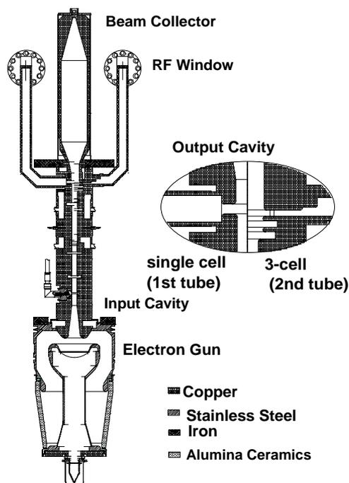
Figure 1: Cross sectional view of E3746 Klystron.
