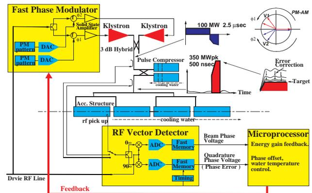
Figure 2: The schematic diagram of the phase modulation system.
