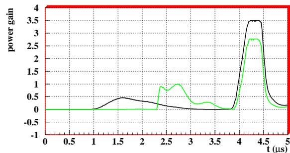
Figure 9: The power gain of the RF-Pulse Compressor.
