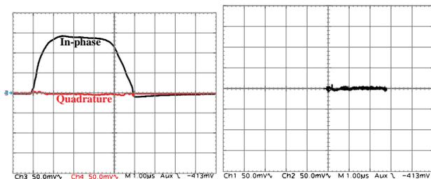
Figure 7: I-Q demodulation pulse with the phase compensation
