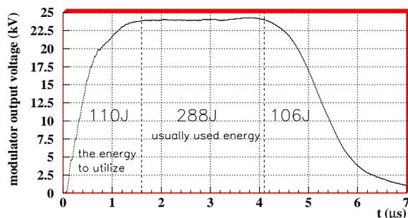
Figure 1: The modulator output voltage on dummy load
