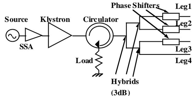
Figure 1: Schematic of LEDA RFQ RF power delivery system.
