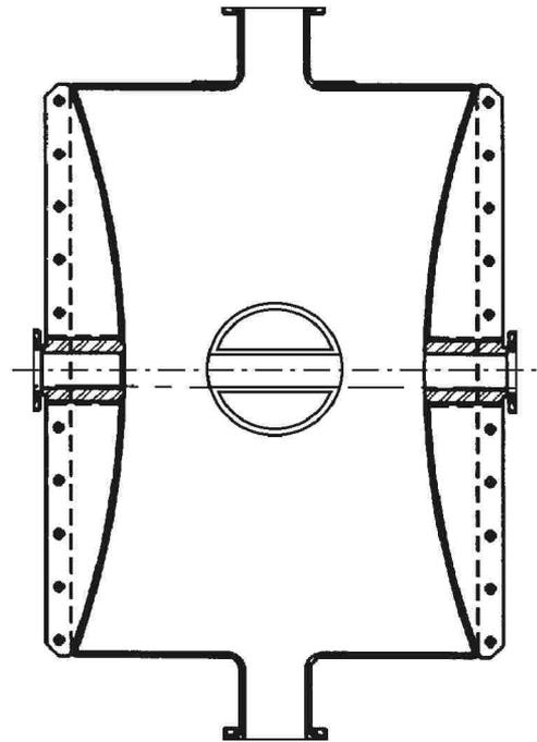
Figure 1: Section for a 44 cm diameter, 350 MHz spoke cavity
