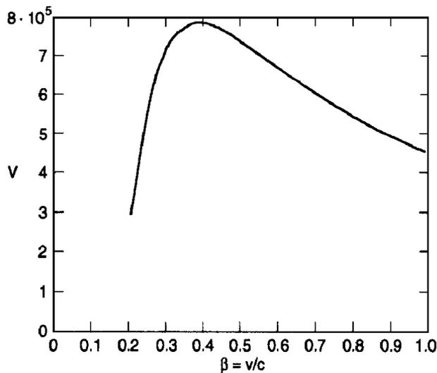
Figure 2: Velocity acceptance characteristic for the two-gap,  $\beta = 0.4$  spoke cavity. The voltage gain is given in volts for an rf energy content of 1 joule, corresponding to an accelerating field of 3.4 MV/m in the 22.9 cm long structure.
