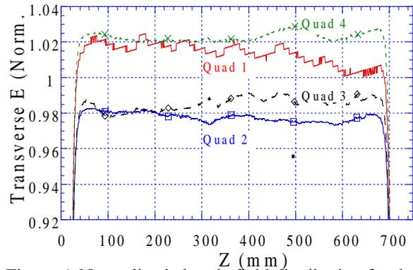
Figure 6. Normalized electric field distribution for the 4 quadrants after 0.1 mm misalignment of one of them
