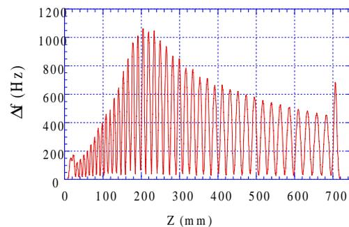
Figure 4:  $\Delta f (\propto E_z^2)$  distribution at beam axis
