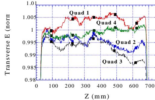
Figure 3: Close view of normalized transverse electric field distribution for 4 quadrants
