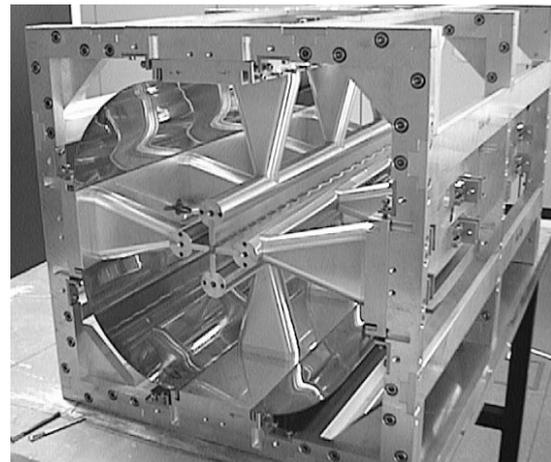
Figure 1: View of the half scale model of SRFQ1 (end flanges and one of the shells are not installed)
