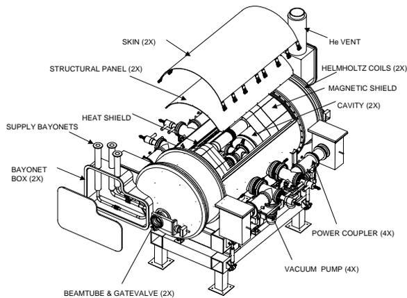
Figure 1: The  $\beta=0.64$ , 2 cavity, ED&D Cryomodule.
