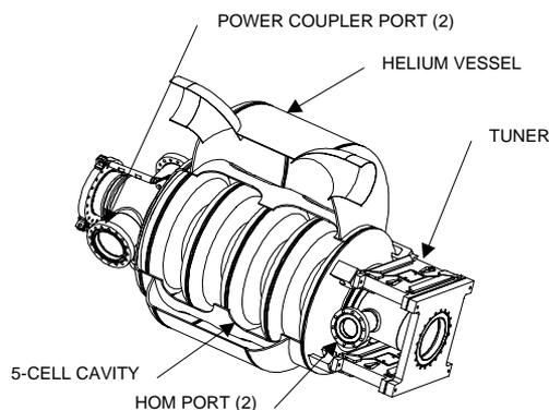
Figure 3: A  $\beta=0.64$  Cavity and Helium Vessel
