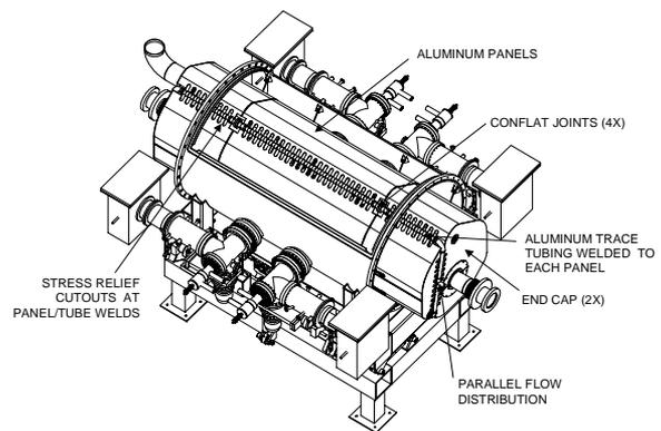
Figure 2: Complete RF Section with heat shield installed.
