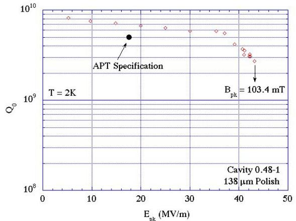
Figure 2: Typical test results of a  $\beta = 0.48$  cavity
