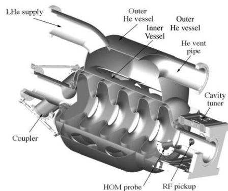
Figure 1: Illustration of  $\beta = 0.64$  cavity design.
